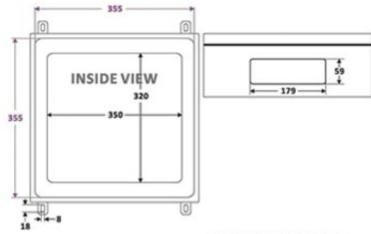
DIMENSIONS ARE IN: MM TOLERANCES: ±2MM
