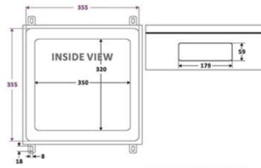
DIMENSIONS ARE IN: MM TOLERANCES: ±2MM
